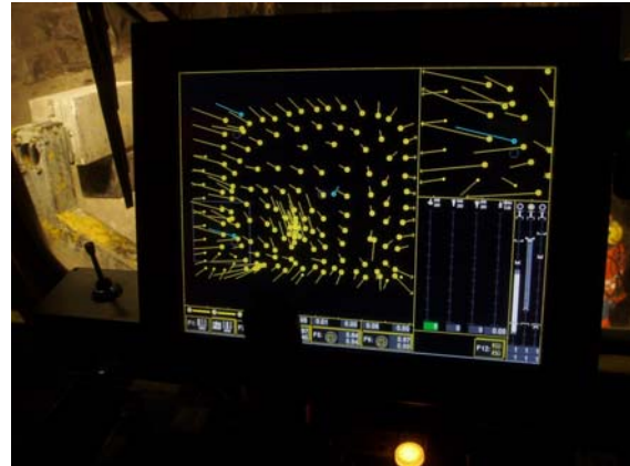
Normal drilling display showing face drill pattern and sequence for automatic positioning
