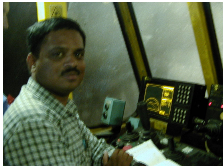
Operator checks overbreak from cabin
